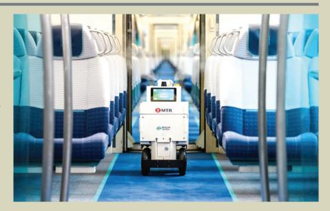
allows for greater manoeuvrability. The robot can be operated automatically or via remote control.
