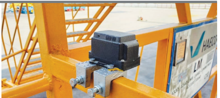
A LoRaWAN tracker is installed on GSE for location tracking. 地勤設備上安裝了遠程低功耗 (LoRaWAN) 追蹤器，以便追蹤位置。
