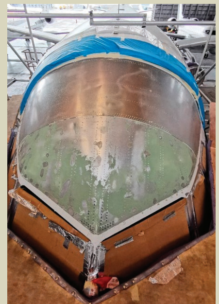
CASL replaces the skin panel of an aircraft. 中飛為飛機更換蒙皮。
